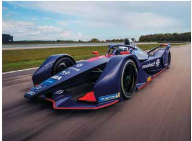
Electric Formula-E racing cars have 250kW of power and will accelerate from 0-100 km/h in 2.8-seconds with a top speed of 280km/h.
